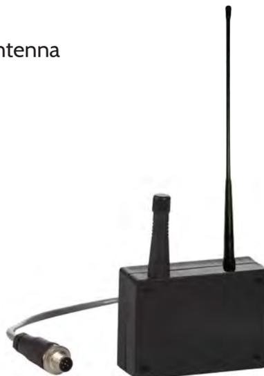
HVDS Node - The HVDS Node gives remote HVDS sensing to the TSafe system. It works as a complete HVDS giving 360° overhead high voltage cable detection and transmits its data (hard-wired or wirelessly) to the TSafe ECU. Up to 3 nodes can be connected to a TSafe system giving 4 High voltage detectors in total.
