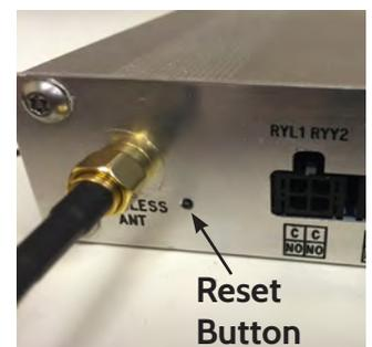
If the number at the side of the add device symbol reads '0' then you will need to briefly press the 'RESET' button located on the side of the ECU. When the reset button is pressed the red status light will stop flashing while the button is depressed. When the reset button is released '1' should appear at the side of the add device symbol showing that the ECU has been recognised as a new device. Press accept to confirm and pair the units.
